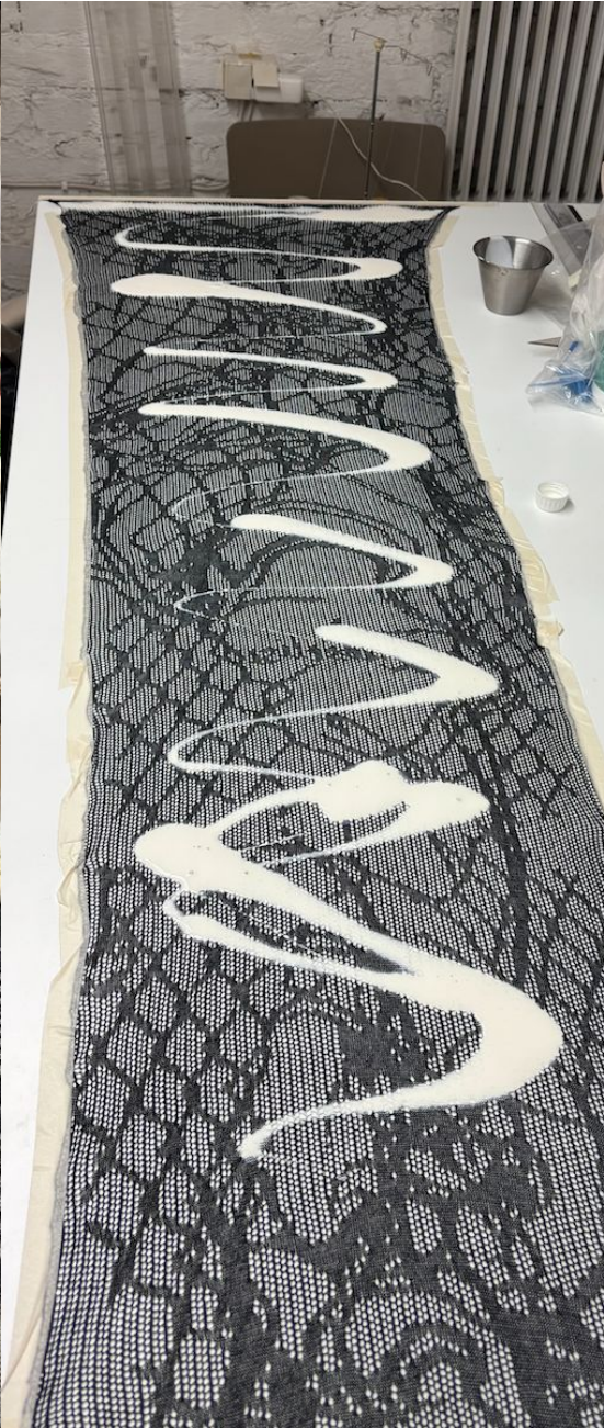
ADF-knit (pointelle structure) + latex coating
