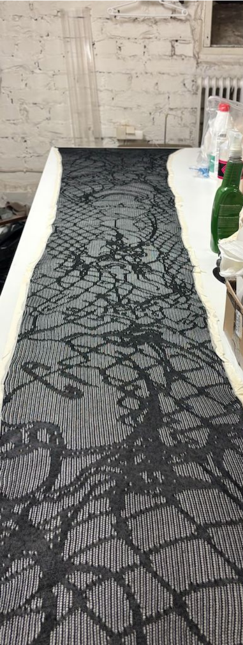
ADF-knit (pointelle structure) + latex coating
