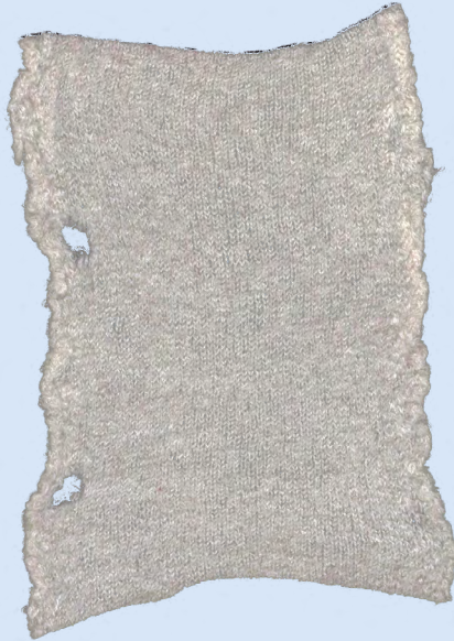
sample 3 | single knit gauge 5, tension 13
