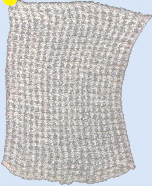
sample 1 | tuck stitch gauge 5, tension 15
