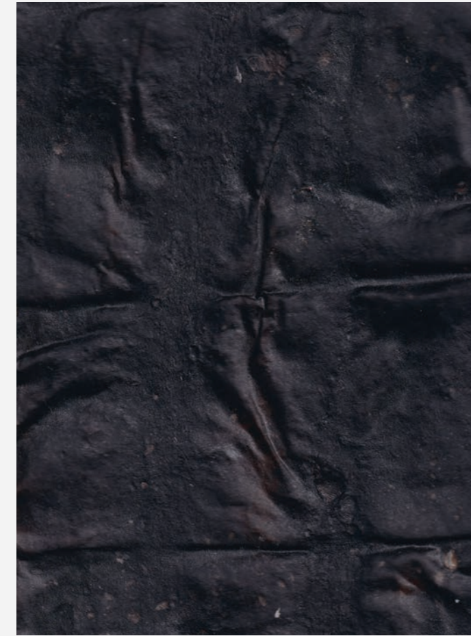
Leather made out of egg carton, glyserol and agar. Dyed with green tea.
