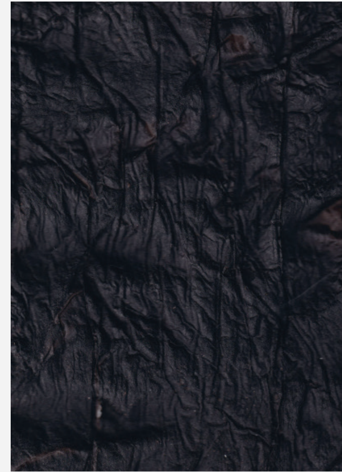
Leather made out of egg carton, glyserol and agar. Dyed with green tea. Wrinkled by drying
