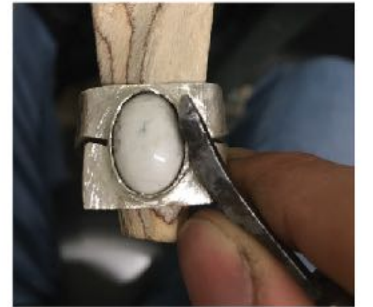
7. Filling and sanding inside of the ring & outside of the bezel; 8. Polishing; 9. Setting stone
