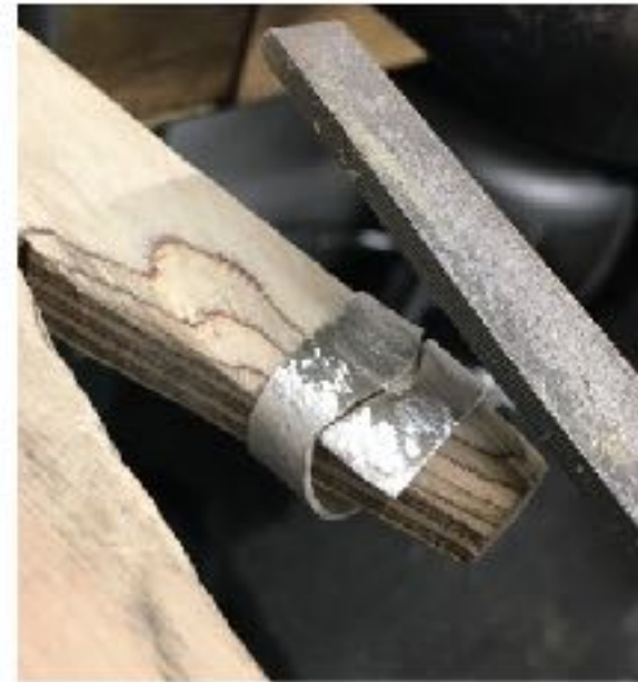
5. Using pliers/ filings to flatten the stone setting area.
