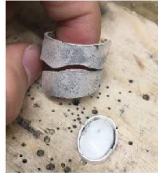
2. Annealing and bending, back and forth
